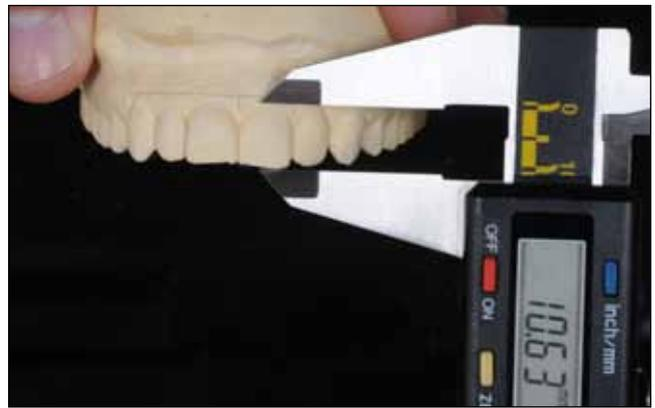
**Fig 12** Measuring the length of the left central incisor (10.6 mm) on the cast. This measurement will be transferred to the computer for calibration of the digital ruler.
